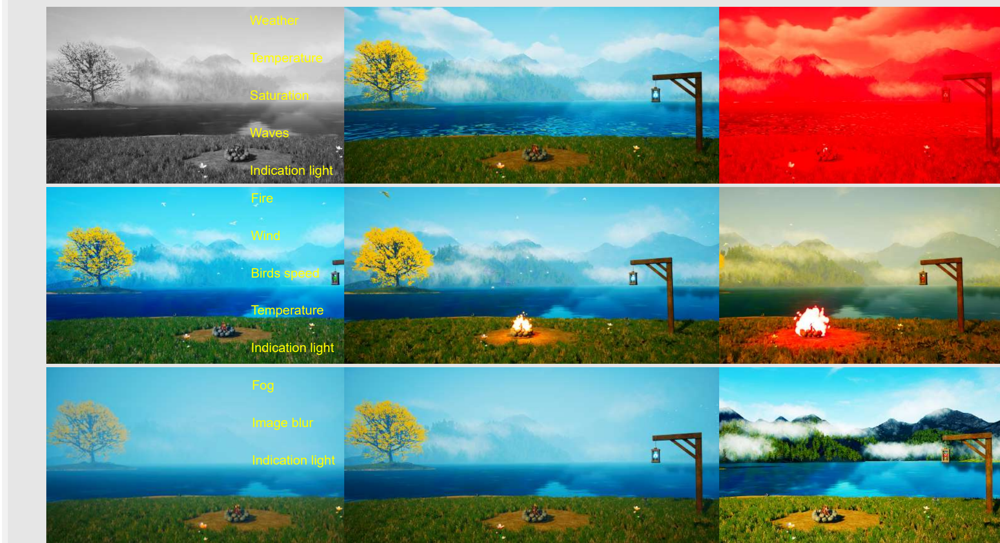
Figure 8: dynamic ambiances and active feedback elements The 3D immersive VR environments are modulated every 5 seconds based on real-time EEG-based arousal estimation over the previous 10 seconds. Feedback elements reflect the user's current arousal state, with the most balanced environment corresponding to the target medium arousal state. To optimize engagement and arousal control, the environments are divided into dynamic ambiances with distinct feedback elements. Transitions between ambiances depend on the user's ability to reach and maintain the target arousal state.
